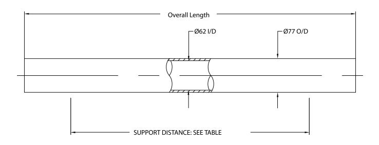
Working Pressure: 1000 psi Working Temperature: -70 to 450 C
